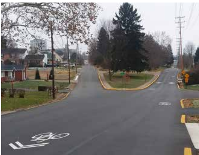
Laurel Street in the Suncrest neighborhood features both shared-lane markings and speed humps
