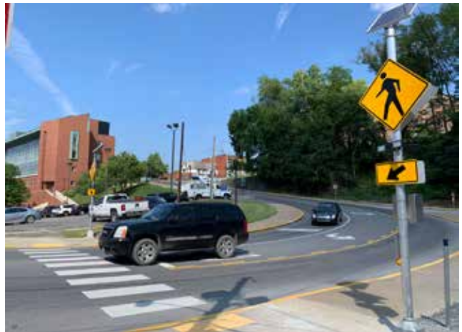
Rapid flashing beacon at the University Avenue crosswalk at Falling Run Road
