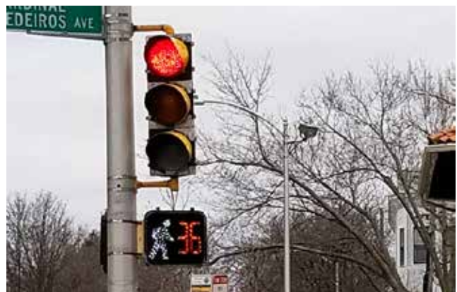
Lead pedestrian intervals give walkers a few seconds head start to cross at a signalized intersection
