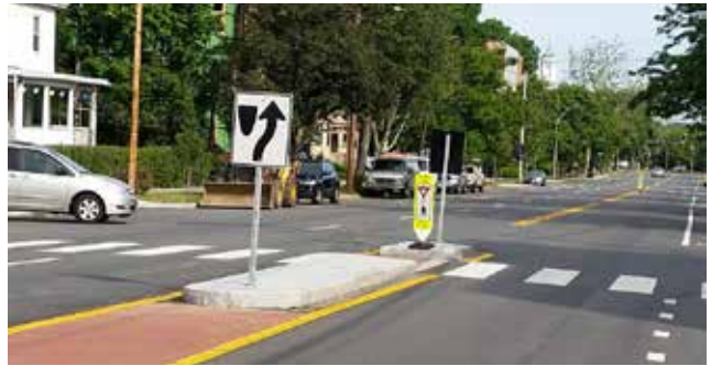
Example crosswalk with median island
