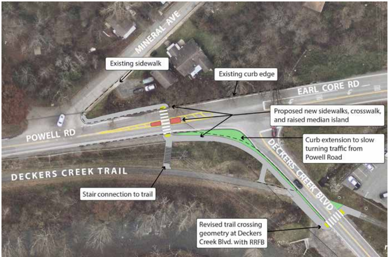
Design graphic showing the approximate location of the recommended crosswalk between Mineral Ave and Deckers Creek Blvd and the improved crossing of the trail
