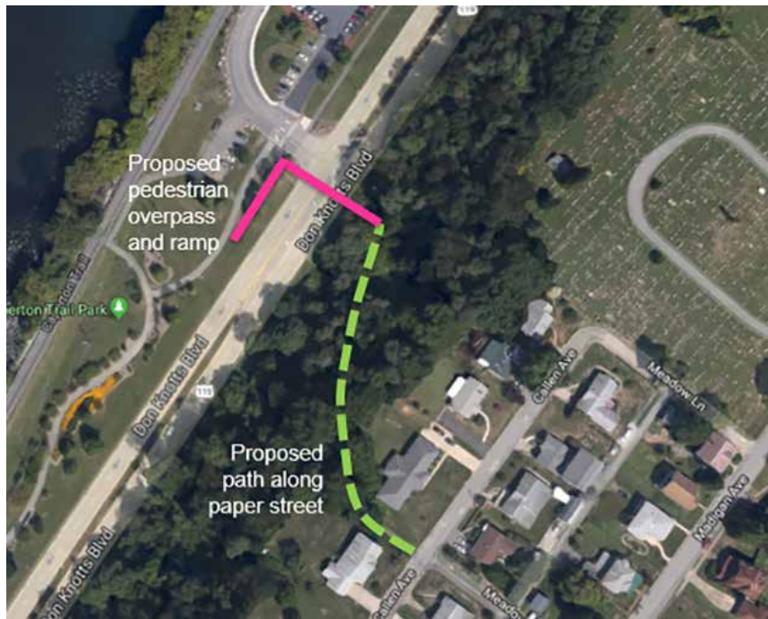
Diagram illustrating the alignment of the pedestrian/bicycle bridge over Don Knotts Boulevard with connections to the 1st Ward neighborhood and the riverfront trail system
