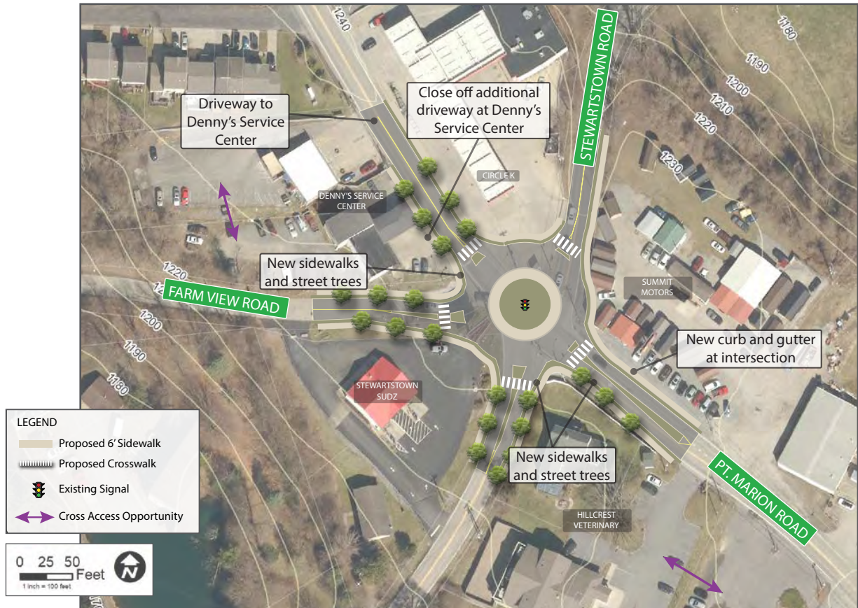
Figure 5.8: Conceptual design of Point Marion Road/Stewartstown Road - 5-leg single-lane roundabout.
