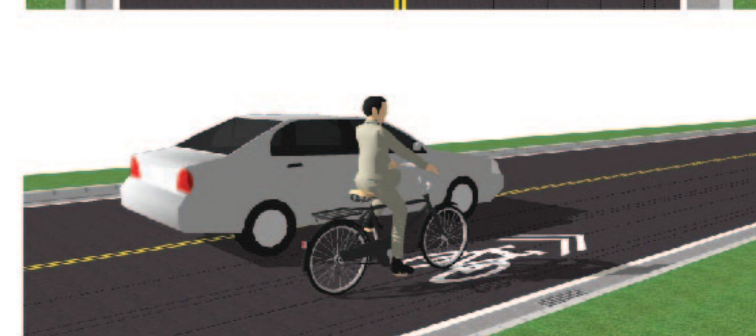
Best Use: Space-constrained roads with narrow travel lanes, or road segments upon which bike lanes are not selected due to space constraints or other limitations.
