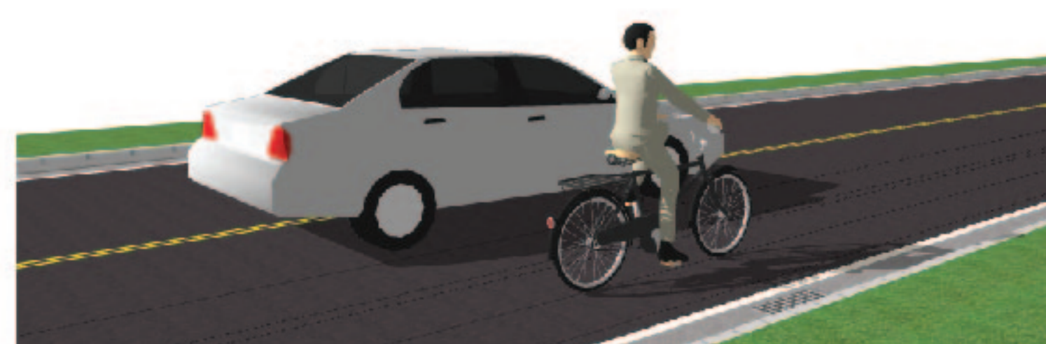
Best Use: Minor roads with low volumes, where bicyclists can share the road with no special provisions.
