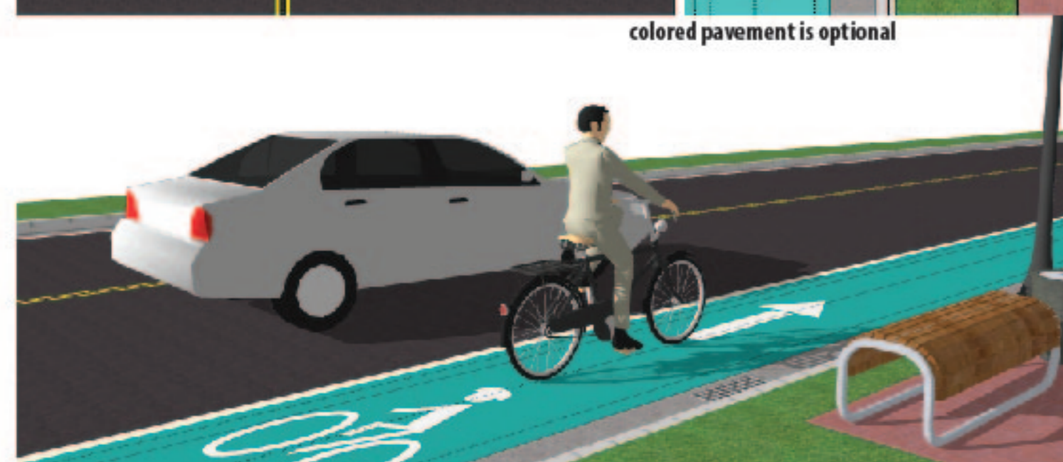
Best Use: Major roads that provide direct, convenient, quick access to major land uses. Also can be used on collector roads and busy urban streets with slower speeds.
